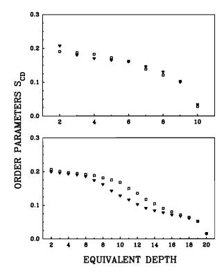
FIGURE 7 Comparison of the  $^2$ H orientational order profiles of 20:12 PC and 10:22 PC as a function of the equivalent depth of the lipid bilayer. The orientational order profiles of the short chains (top) and long chains (bottom) are compared at  $T_{\rm m} + 6^{\circ}$ C. The filled symbols define the order profiles of 10:22 PC, and the open symbols define the order profiles of 20:12 PC.
