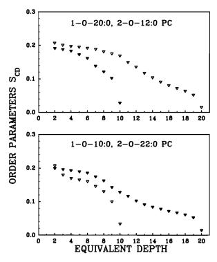
FIGURE 6 Comparison of the  $^2$ H orientational order profiles described by the long and short chains of 20:12 PC (top) and 10:22 PC (bottom) as a function of the equivalent depth of the lipid bilayer. The open symbols describe the orientational order profiles of the sn1 fatty acyl chains, and the closed symbols describe the orientational order profiles of the sn2 fatty acyl chains. The data shown were all acquired at  $T_m + 6$ °C.
