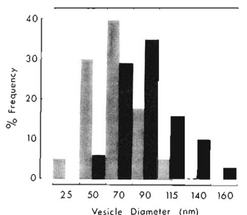
Fig. 3. Size distribution of soya PC vesicles obtained after 10 extrusions through a polycarbonate filter with 100 nm pore size. The vesicle diameters were measured from freeze-fracture micrographs employing the technique of Van Venetić et al. (1981). The half-tone columns represent vesicles that did not undergo a freeze-thaw cycle, the black columns represent vesicles subjected to the freeze-thaw protocol outlined in Materials and Methods.
