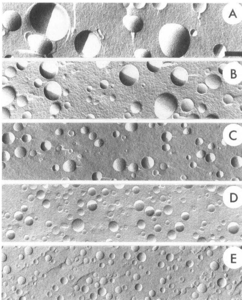
**Figure 1.** Freeze fracture electron micrographs of EPC frozen and thawed MLVs (100 mg/ml) extruded 10 times through polycarbonate filters with pore sizes of 400 nm (A), 200 nm (B), 100 nm (C), 50 nm (D), and 30 nm (E). All micrographs were obtained under the same magnification; the bar in A represents 150 nm.
