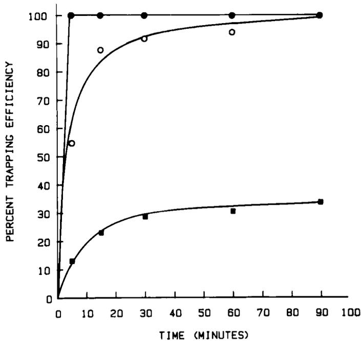
**Figure 2.** Uptake of doxorubicin (3 mg/ml) into EPC/cholesterol (55:45, mol/mol) liposomes (11 mg/ml) exhibiting a pH gradient (pH 4.0 inside, 7.5 outside) at 21°C (■), 37°C (○), and 60°C (●).
